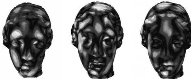
Fig. 14. Error distributions. The simplified Venus model is composed of about 300 triangles. Left: QSLIM, middle: JADE, right: proposed algorithm
